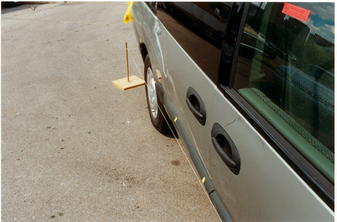
45. View of the right side direct contact damage.
